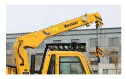
**OPTIONAL CRANE.** Choose the optional telescoping crane to help reduce the amount of support equipment needed onsite.
