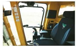
**OPERATOR'S STATION.** Operator comfort was top-of-mind with the design of the FT300. Standard air-ride seating, ergonomic controls and optimal viewing allows for less strain on the operator and more focus on production.
