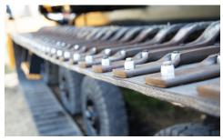
TRACKS. No two jobsites are alike which is why the FT300 offers two track options. A 30" (76.2 cm) wide single grouser steel track is ideal when superior tractive effort is needed while a 33" (83.8 cm) wide low ground pressure (LGP) track offers a light footprint for soft conditions.
