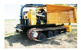
**ENGINE ACCESS.** Two large, hinged doors swing open to expose the sides, top and rear of the engine compartment without additional tools.
